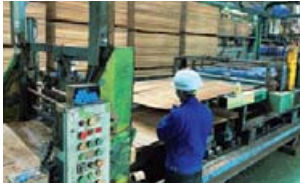
3mmの薄板が積層されLVLとなる 3mm veneers are laminated into LVL
