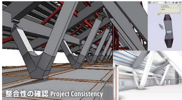
BIMモデルの重ね合わせにより、建築計画・構造計画の整合性を高める Enhancing Conflict Resolution between Architectural and Structural Planning through Overlayingf BIM
