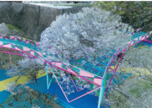
BIMデータと樹木や既存地盤面も含めた城内3次元測量データを統合したもの。施工段階でも活用。 Integration of BIM data and three dimensional survey data of castle grounds. This also proved highly useful during construction.
