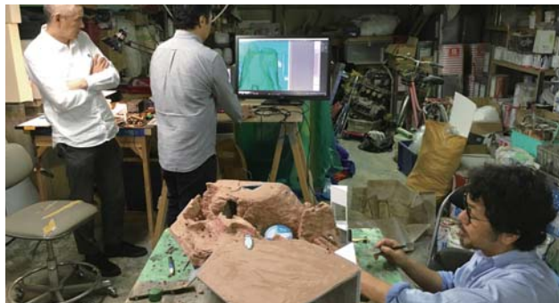
日本海大水槽の擬岩形状の打合せでは、模型と3Dソフトで並行して納まりや展示効果を検証。 The Artificial Seafloor in the Sea of Japan Giant Water Tank Was Analyzed with Models and 3D Software Modelling to Confirm Fit and Exhibit Effects
